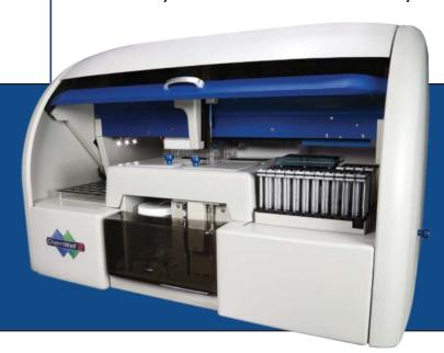
ChemWell-2 is a two-plate ELISA analyzer, capable of simultaneously processing two standard microwell plates or 8-well microwell strips in microwell strip carriers. The flexible analyzer can run multiple assays on each of the microwell plates automatically adjusting for timing, incubation, wash, and rinse cycles.
